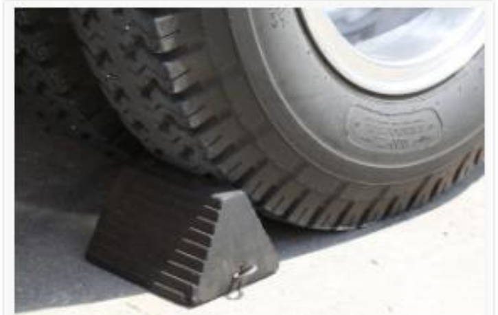
A pyramid style wheel chock used to prevent the wheels from unintentionally moving.
